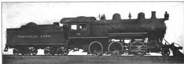
Fig. 35. Mogul (2-6-0) Locomotive. Built by the American Locomotive Co. for the Vandalia Line. Cylinders 21 in. x 28 in., Working Steam Pressure 200 lbs per sq. in., Total Heating Surface 2,935 sq. ft., Diameter of Drivers 63 in., Weight on Drivers 156,500 lbs., Total Weight 182,500 lbs.
